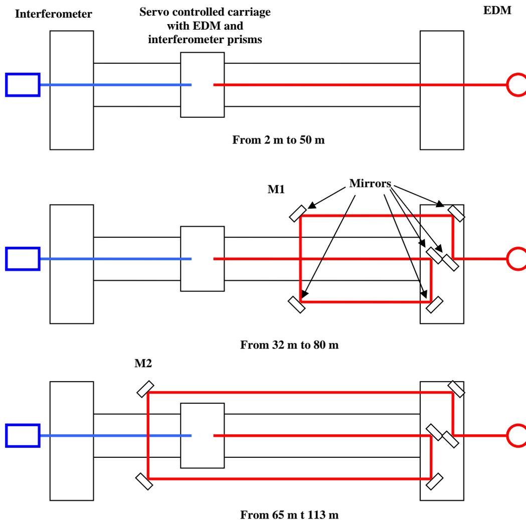
**Figure 4** Schematic view of the 1.9m to 50m and 1.9m to 113m EDM calibration technique. For the 113m calibration, first a 50m calibration is performed. Second two mirrors (M1) are used for comparative overlapping measurements between 32m and 80m. Third mirrors M1 are move out of the way and measurements are made between 65m and 113m using mirrors M2.
