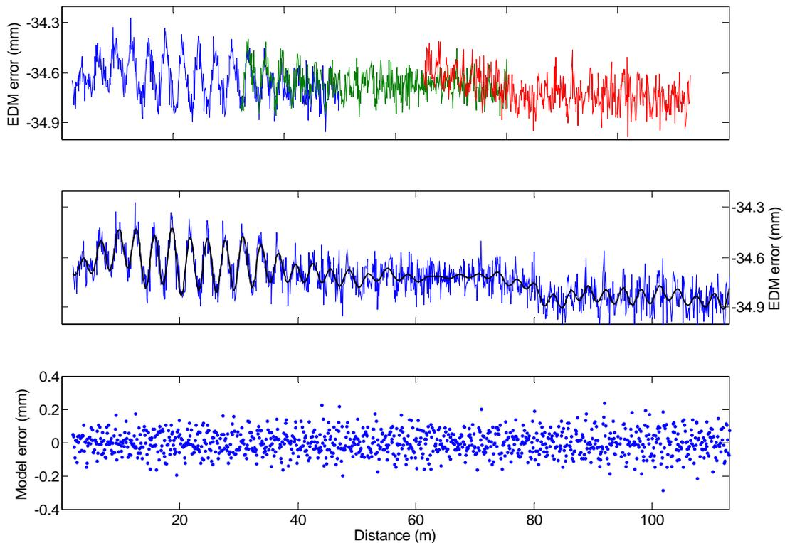
**Figure 1** Typical 113m EDM calibration curve. The top graph shows results for the three sections of the calibration: 2m to 50 m, 32m to 80m and 65m to 113m. The middle curve shows the calibration results and a best model. The bottom curve shows residuals with respect to the model curve. The overall standard deviation with respect to the model curve is 0.07 mm.
