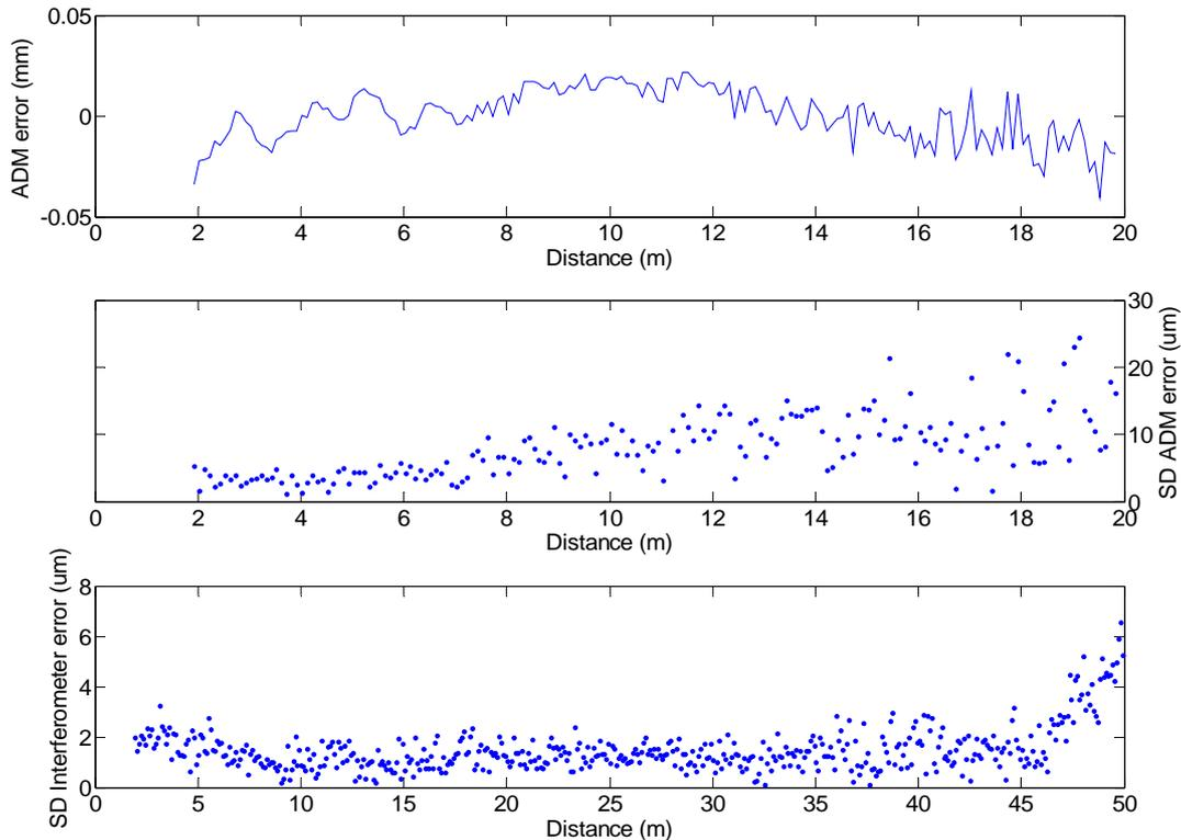
**Figure 3** The top graph shows calibration results for a laser tracker ADM as between 1.9m and 20m. The middle graph shows the standard deviation (i.e. repeatability) for the 4 calibration series of laser tracker ADM. The overall standard deviation is 20 µm. The bottom graph shows the standard deviation of the laser tracker IFM (interferometer) between 1.9m and 50m for 4 calibration series with the same laser tracker. The overall standard deviation is 2 µm.
