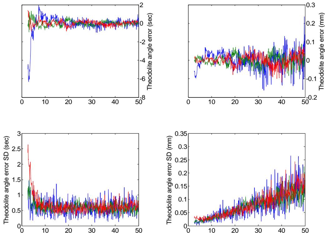
**Figure 2** Results of angle dependence on distance for three RTS instruments of the same model type. Each instrument was calibrated 15 times. The top left graph shows the error with respect to the mean angle reading in arc seconds. The top right graph shows the same but reduced to an offset distance (i.e.  $y = d \sin \alpha$ ). The bottom graphs show the standard deviations for the fifteen measurement series in arc **seconds (left)** and **mm (right)**.
