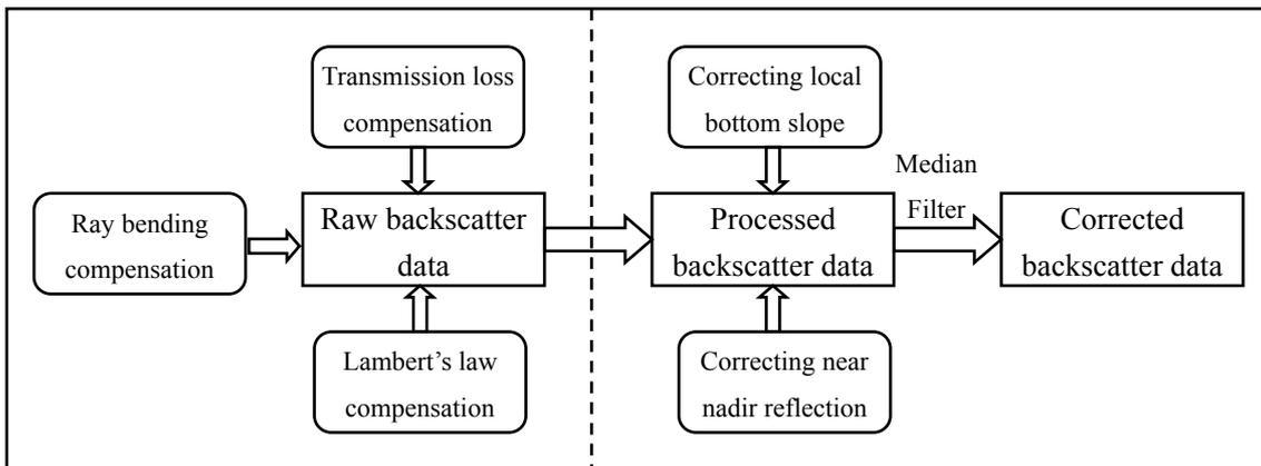
**Figure 2** Process flow for backscatter data pre-processing
