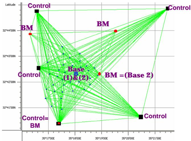
**Figure 3:** The whole measured vector's picture including the description of the two RTK bases location points. The BM indicates a licensed vertical Control network with high grid 1, and the control is a control point with licensed coordinates in high order level (3).
