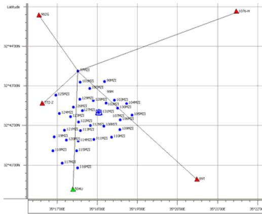
**Figure 1:** The 35 control points control network and an example for linking every point to the national control grids.
