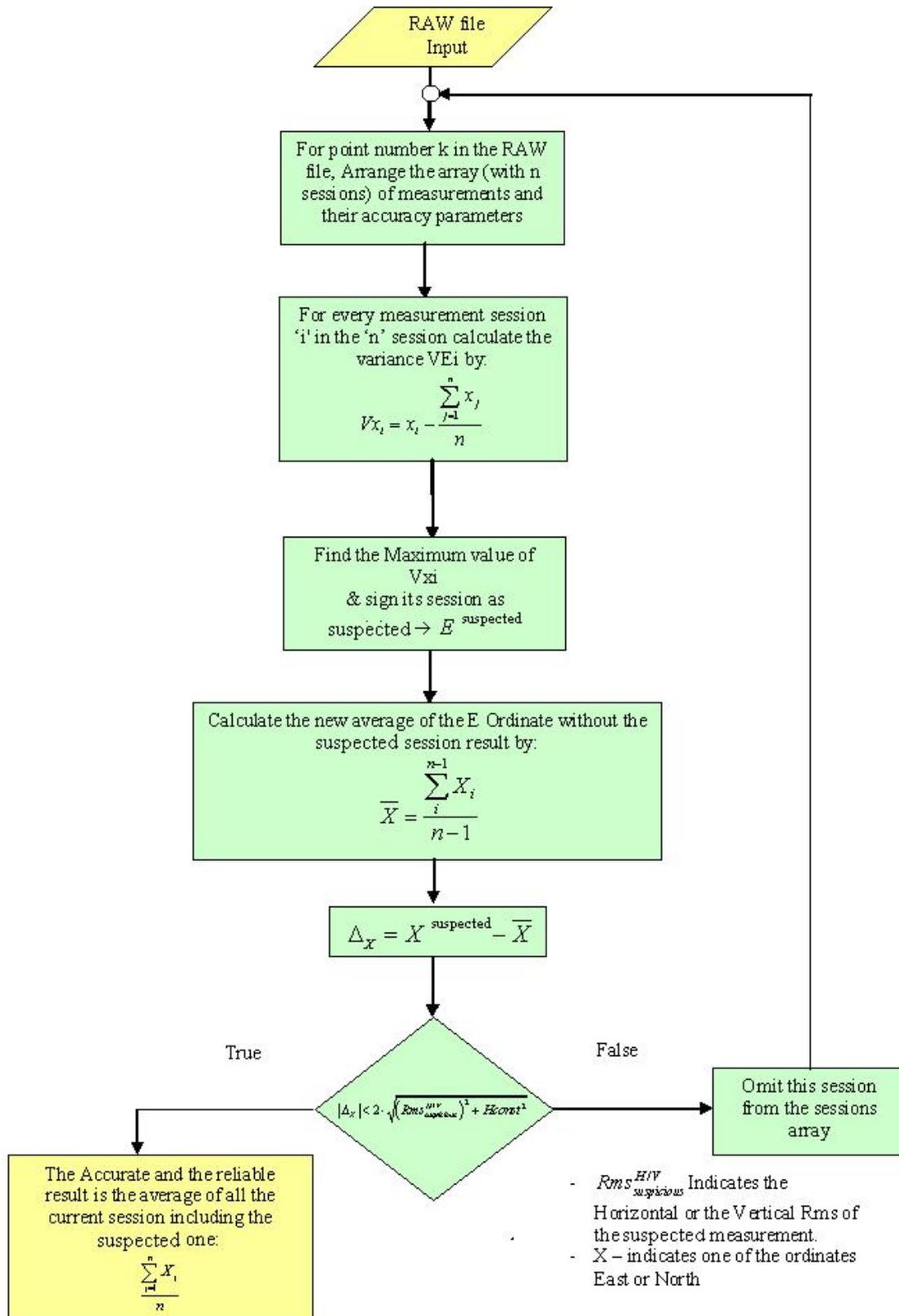
**Figure 4:** An algorithm Dealing with unstable condition in ROB method
