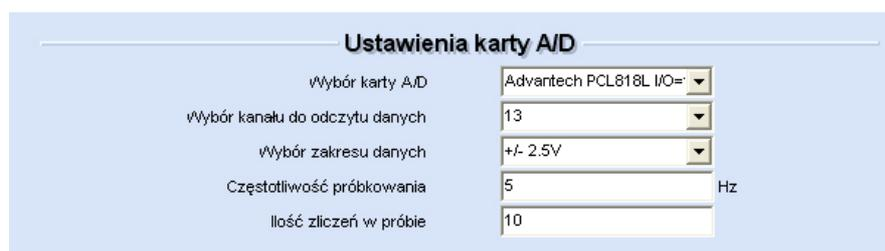
**Fig. 1.** Settings screen in AutoL&R 'A/D Card Settings' section.
