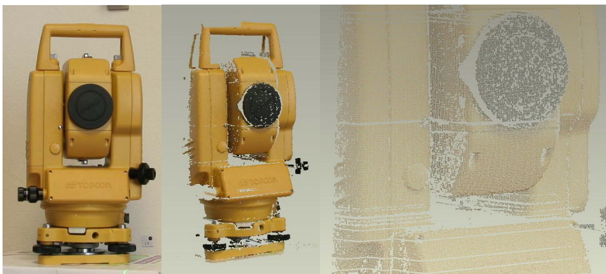
Figure 9 – Photo, point cloud and point cloud detail of Topcon GPT 2006
