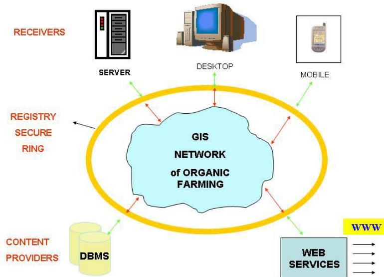
**Figure 4:** Components and Information Flow of a prototype Web based GIS system with a secure ring where needed.
