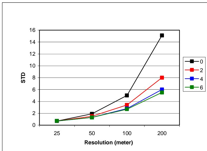
**Figure 7:** Bilinear Profiles Method – STD (meter) figures of the southern area – full coverage
