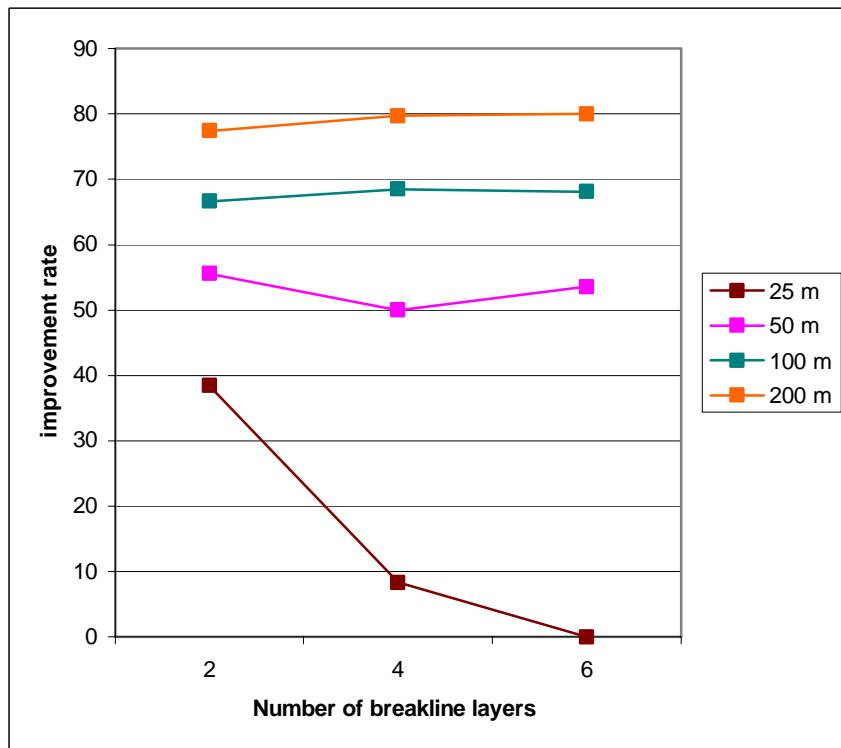
**Figure 10:** Bilinear Profiles Method - STD improvement rates of the southern area – 10-meter buffer
