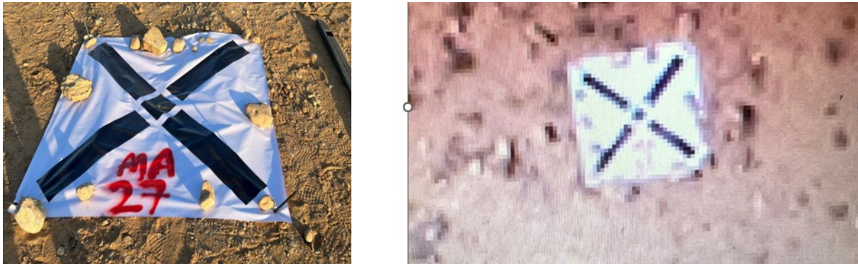
Figure 1. GCP marked on the ground (left) and GCP as seen in imagery (right).
