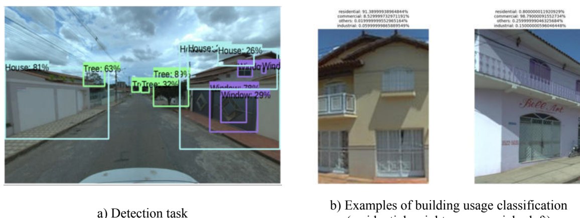
Figure 1. Example of automated building detection (a) and classification (b) using 360° terrestrial mobile mapping imagery in an urban environment.
