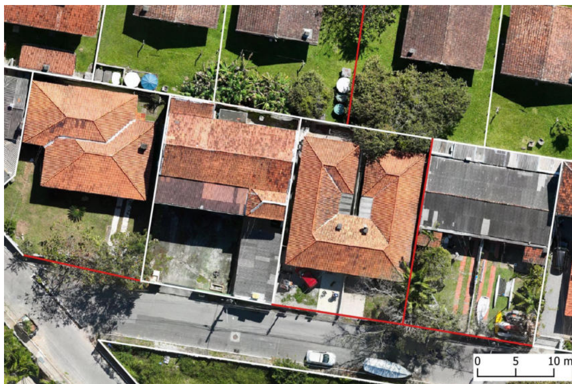
Figure 11. Vectorization of parcel boundary lines.
