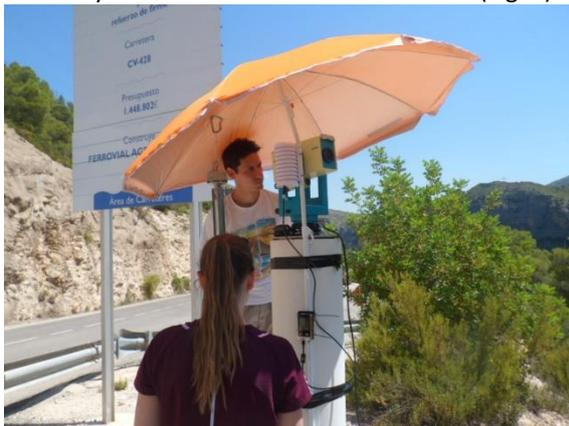
Figure 6. Distance measurement with the ME5000 Mekometer. Both traditional and digital meteorological sensors were simultaneously used at the EDM end.
