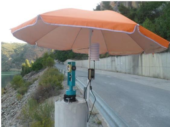
Figure 5. Pillar equipped with a parasol and a data-logger for dry and wet temperatures as well as air pressure.
