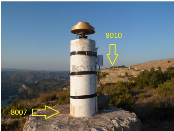
Figure 8. Leica AR25.R3 choke-ring antenna set up at dusk for GNSS distance measurement between pillars 8007 and 8010, which do not have straight sight between them.
