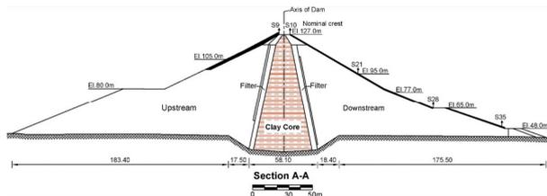
Figure 1(b). Maximum cross-section along A-A (after Michalis et al., 2016)
