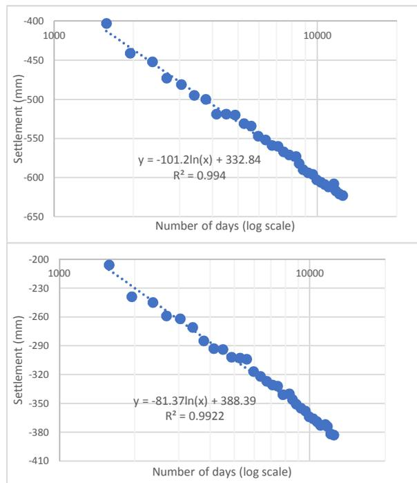
Figure 9 Settlement vs number of days for control station (a) S9, and (b) S10.
