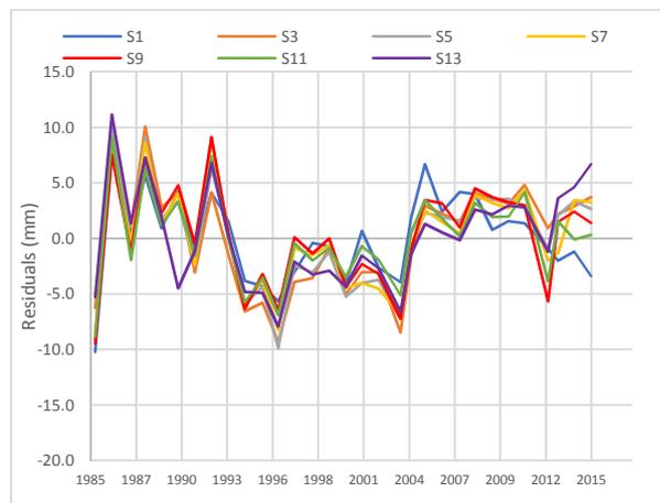
Figure 10(a). Residual settlements for control stations S1 – S13 along the upstream side of the crest
