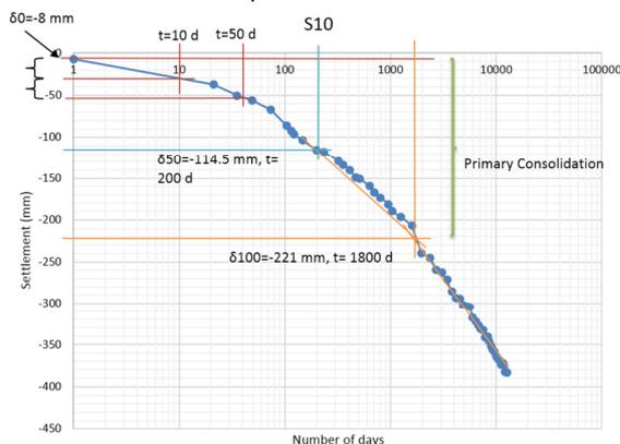
Figure 4(b). Vertical Settlement vs Number of Days (log scale for the x-axis) for control station S10
