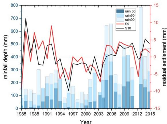
Figure 13. Cumulative rainfall and settlement residuals for control points S9 and S10
