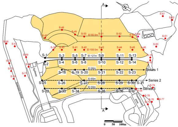
Figure 1(a). Plan view of Pournari I Dam and its geodetic monitoring network. This study only uses observations for points S1-S14, located along the crest (after Michalis et al., 2016).
