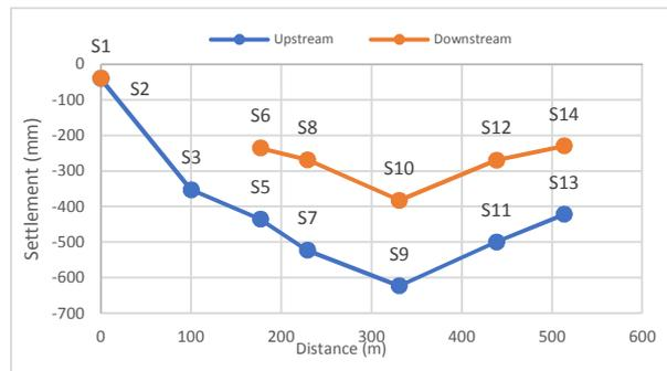
Figure 8. Observed settlement along the dam's upstream (blue) and downstream (orange) side of the crest on 01/04/2015
