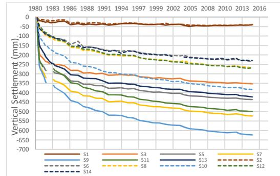
Figure 2. Recorded settlements for the 13 control stations on the crest between 1981 and 2015. For location of these stations, see Figure 1(a).
