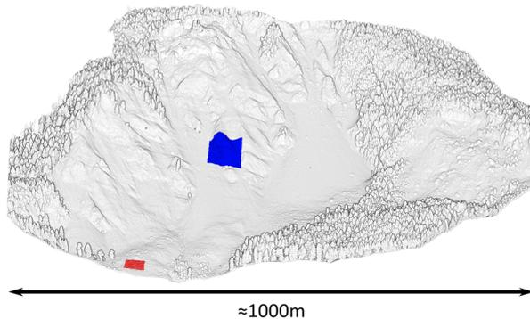
Figure 8: Reference point cloud of the landslide located in the Swiss Alps acquired using a drone based LiDAR system. We perform the deformation analysis for the areas marked with the red (Area 1) and blue (Area 2) color.
