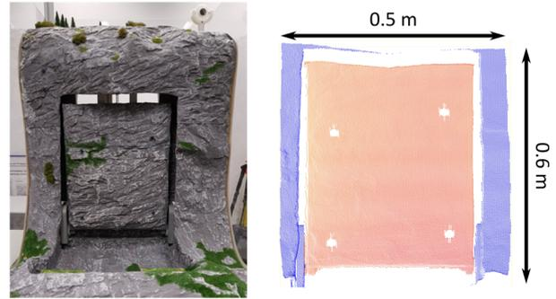
Figure 3: Rockfall simulator (left) and a point cloud acquired using a Leica MS50 (right). Red color shows the moving part and the blue color the stable part of the simulator. Holes in the red part of the point cloud show the location of the four mini prisms.
