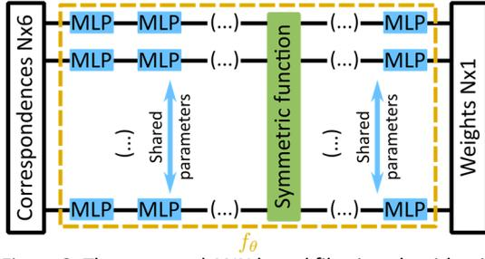
Figure 2: The proposed ANN based filtering algorithm is composed of several MLPs operating on individual correspondences and symmetric functions aggregating local information across the whole input. The parameters of MLPs are shared for all correspondences. In the inference phase, the branches are simply copied to fit the number of points in the input
