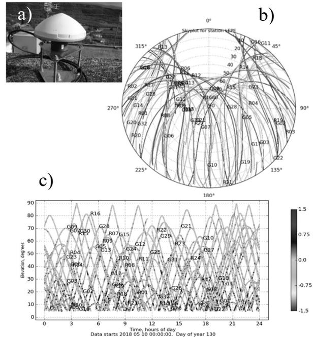
**Figure 4:** a) Antenna installation in station LEPE, b) skyplot example and c) time-elevation plot example of multipath, for station LEPE
