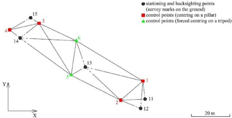
Fig. 1 Geodetic control network
