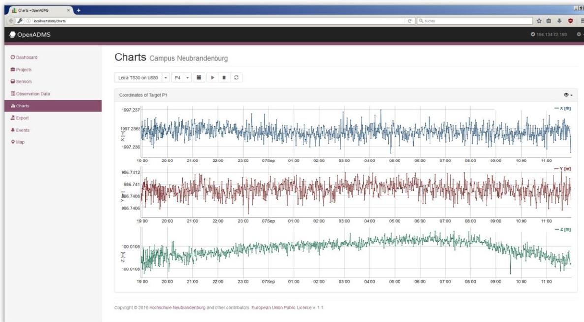
Fig. 3 OpenADMS Web application for remote control of sensor networks
