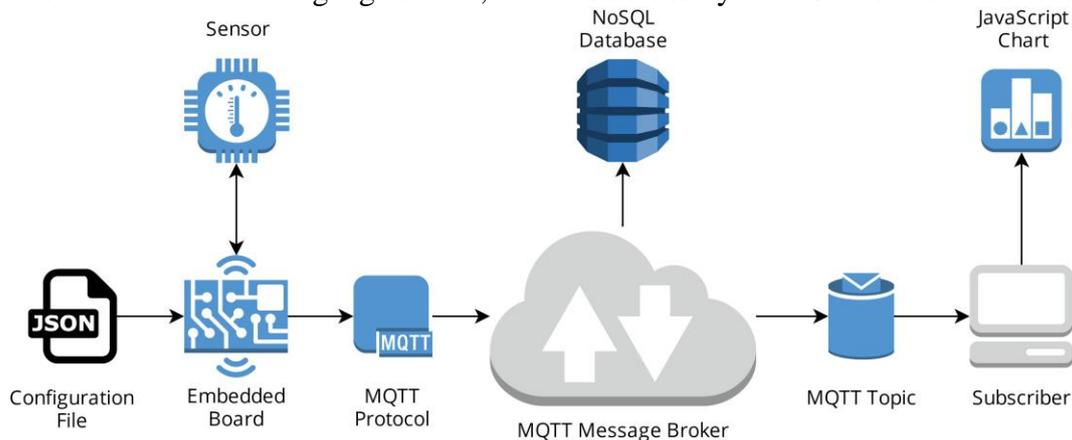
Fig. 2 Distributing observation data in JSON format with the MQTT protocol
