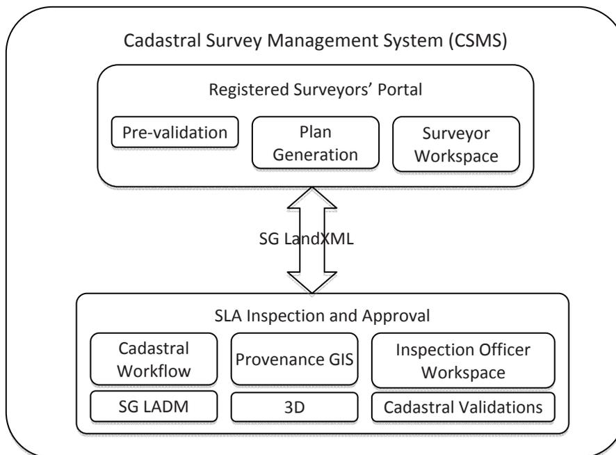
**Figure 3. The design architecture of Cadastral Survey Management System, CSMS**
