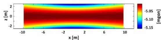
**Fig. 3** Error of horizontal angle  $t$  due to an inclination error of the mirror of  $\Delta\phi = 2.5 \text{ mgon}$  when scanning a plane in 10m distance where the laser scanner is stationed symmetrically in front of the plane.
