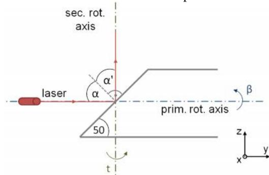
**Fig. 1** Internal construction of a panoramic terrestrial laser scanner.
