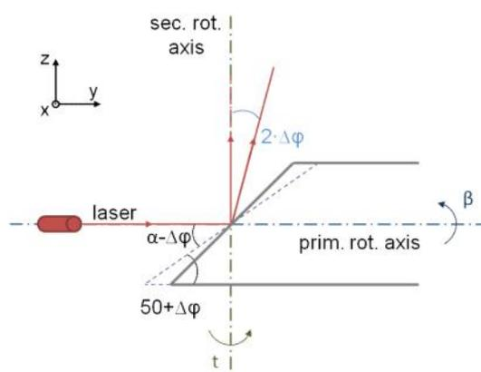
**Fig. 2** Effect on the beam deflection due to a inclination error of the mirror  $\Delta\phi$ .
