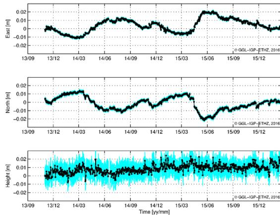
**Fig. 5** Daily solutions of relative displacements in East, North and up directions, between the GNSS stations AL01 and AL02 (AL02 with respect to AL01). The blue bars indicate the uncertainty interval of 3 times the standard deviation.
