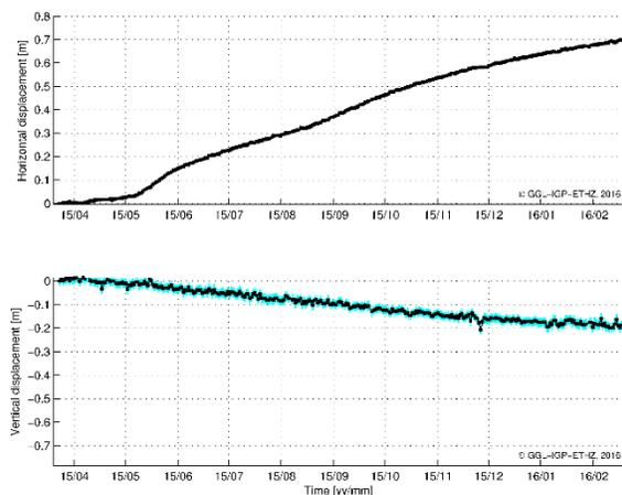
**Fig. 6** Daily solutions of displacements in horizontal and vertical directions. The blue bars indicate the uncertainty interval of 3 times the standard deviation.
