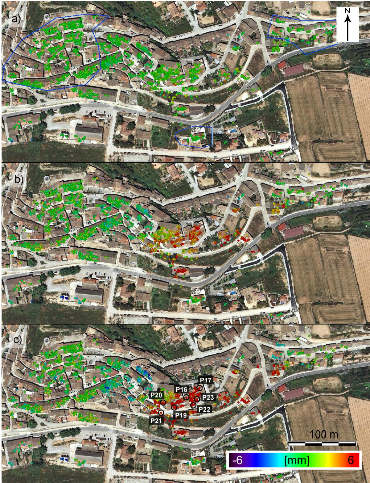
Fig. 1. Displacement maps of Barberà de la Conca between 14/11/2011 and 19/12/2011 (a); 14/11/2011 and 08/05/2012 (b); and 14/11/2011 and 20/03/2013 (c). The blue polygons on the top indicate the stable areas. Figure from Crosetto et al. (2014).
