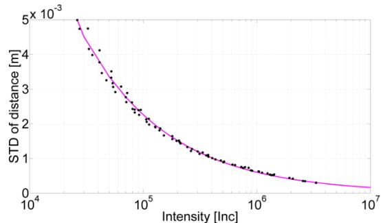
Fig. 1 Intensity vs. precision of a distance measurement
