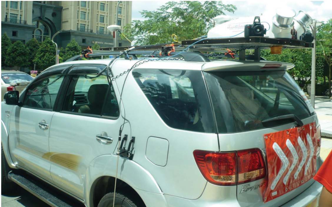
Figure 1: MTLS Dual Laser DynaScan 3 system used
