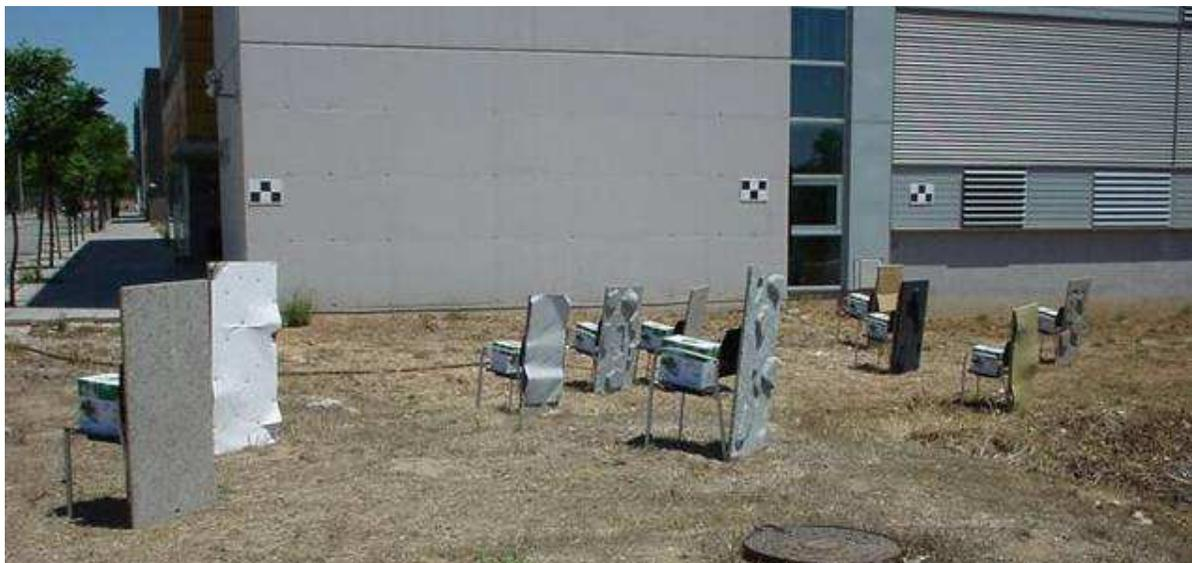
Figure 3 - Image of the targets used to simulate the deformation scenario.
