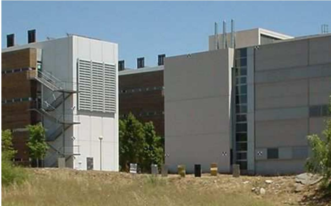
Figure 2 - Image of the experiment. The buildings and structures visible in the photo have been used as stable areas. In the bottom part of the image are located the 10 rectangular artificial targets used to simulate the deformation.
