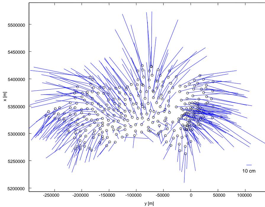
Figure 3 - Residuals of the second transformation without a common scale factor (6-parameter-transformation).
