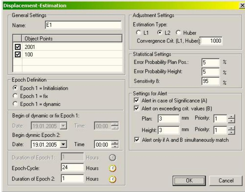
Figure 4: Settings for the GOCA online displacement estimation and alerting.
