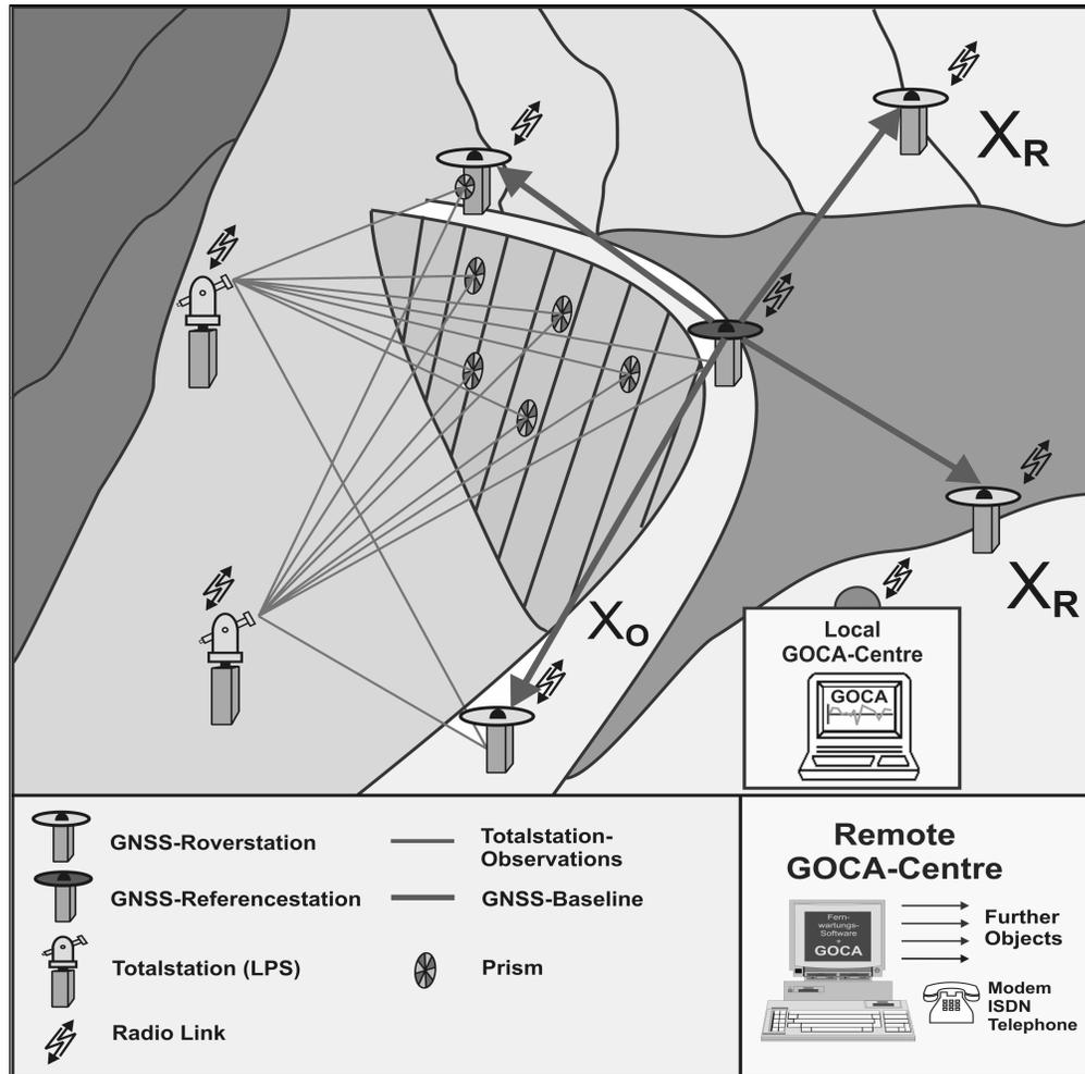
Figure.1: A classical deformation network (stable reference points  $\mathbf{x}_R$  and moving object points  $\mathbf{x}_O(t)$ ) set up online by using GNSS and LPS sensor data in the GOCA system. With the GOCA software several local objects can be monitored simultaneously in a unified reference frame.
