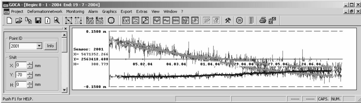
Figure 3: GOCA object-point time series  $\mathbf{x}_O(t_i)$  as result of the 2<sup>nd</sup> adjustment step. The thick lines show the smoothing by a moving average estimation (MVE).
