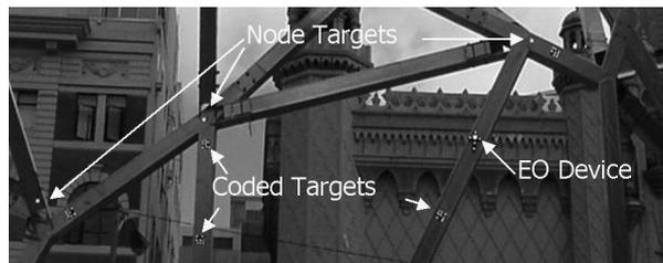
Figure 5. Section of frame showing node point targets, coded targets and an exterior orientation (EO) device.
