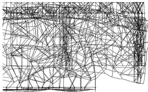
Figure 4. Deflected shape due to dead load in cantilever section (not to scale).
