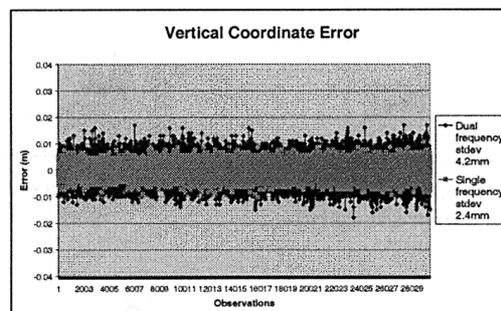
Figure 3 The coordinate error in the vertical direction for the zero baseline tests
