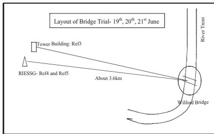
Figure 4 The layout of the 3 remote reference receivers in relation to the Wilford Bridge
