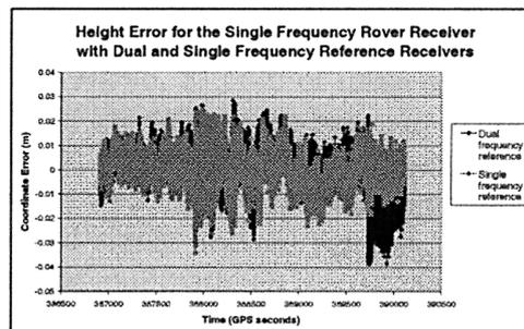
Figure 2 The height error for the single frequency rover processed with dual and single frequency references.
