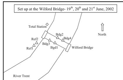
Figure 5 The layout of the receivers at the Wilford Bridge site (not to scale)
