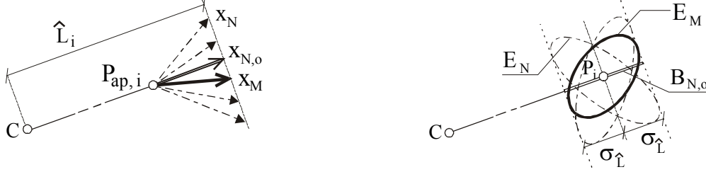
Fig.5 The distance CP_i (a) and its standard deviation \sigma_{\hat{L}} (b) as invariant to the choice of orientation constraint
