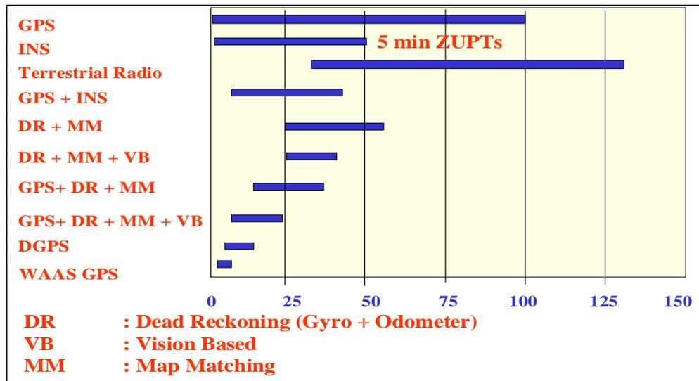
Figure 3: Performance Comparisons of Various Integrated Systems
