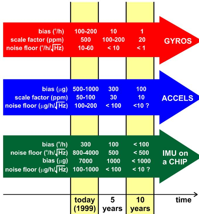
Figure 4: Predicted Development of MEMS-Based Inertial Sensors
