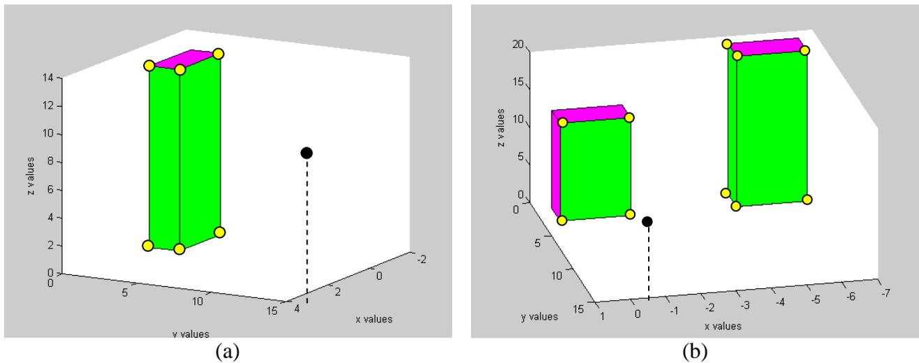
**Figure 4:** Visibility Volume computed with the Analytic Solution. Viewpoint is marked in black, visible parts colored in green, and invisible parts colored in purple. VBP marked with yellow circles - (a) single building; (b) two non-overlapping buildings.
