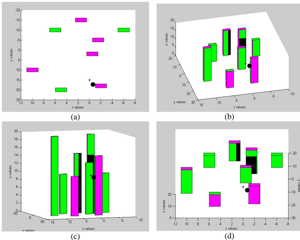
**Figure 8:** Scene number 1: Eight buildings in an Urban Environment,  $V(x_0, y_0, z_0) = (0, 15, 10)$  - (a) Topside view; (b)-(d) Different views demonstrating the visibility computation using our algorithm. CPU time was 0.18 sec.
