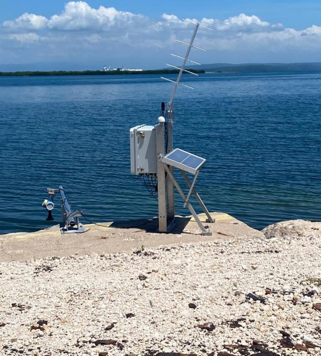
Rocky Point station fitted with **waterlog sensors**, in addition to **submersible sensors**.
