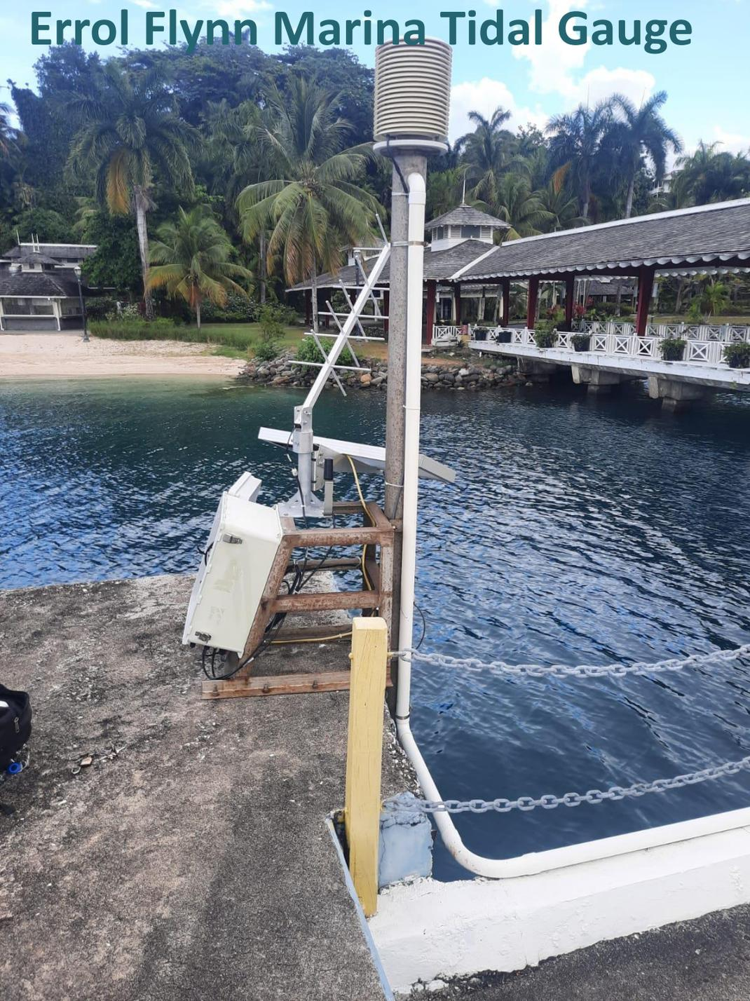
The Errol Flynn Marina has an **acoustic** and **Radar sensor**. The tall pole is the acoustic and radar sensor overhang the water.
