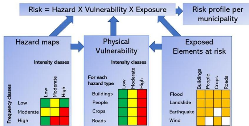
**Fig. 2.** Methodology for analyzing the multi-hazard risk analyses.
