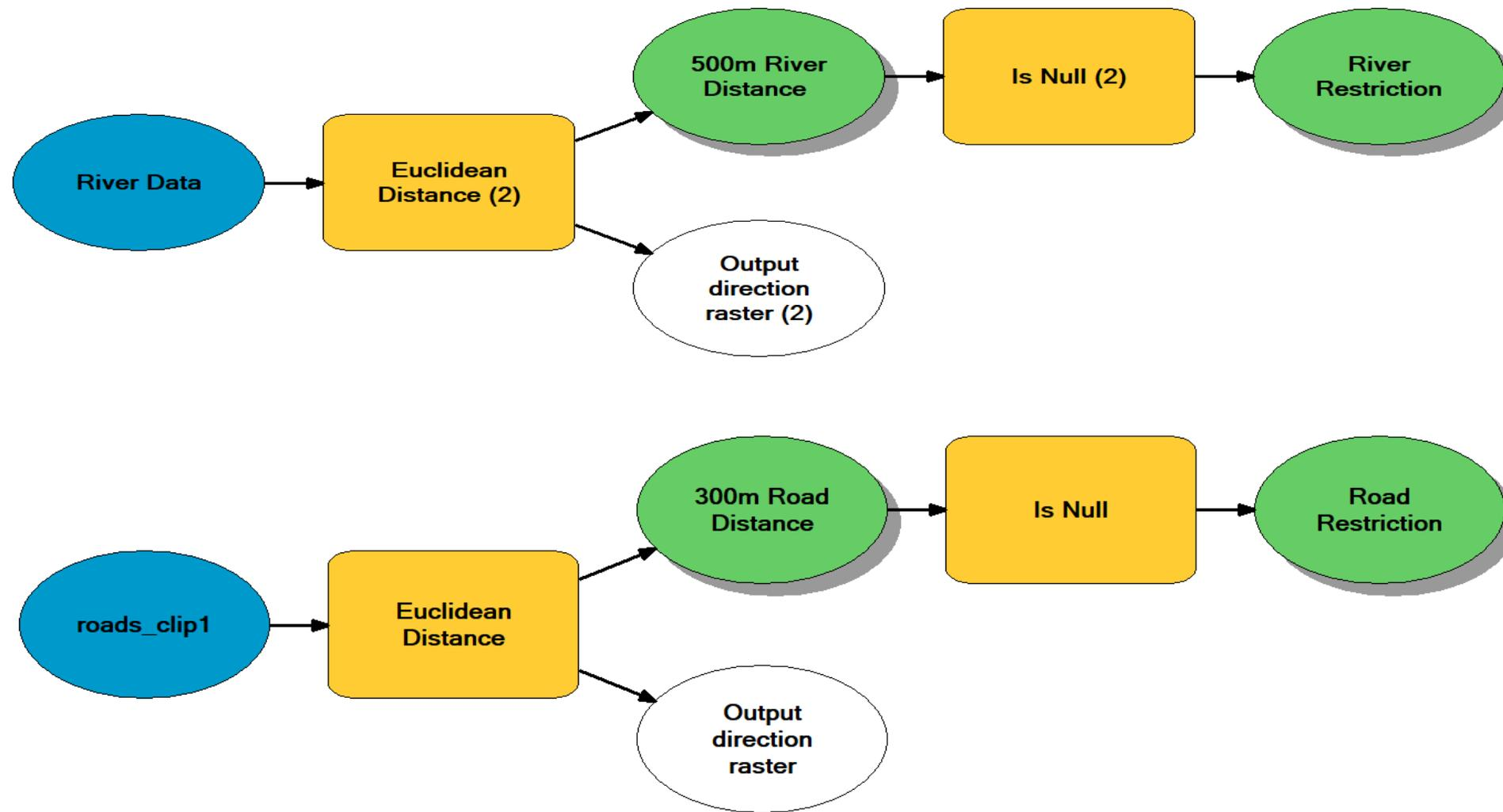
**Fig 5b Site Screening Models for Roads, Rivers and Similar Line-based Criteria**
