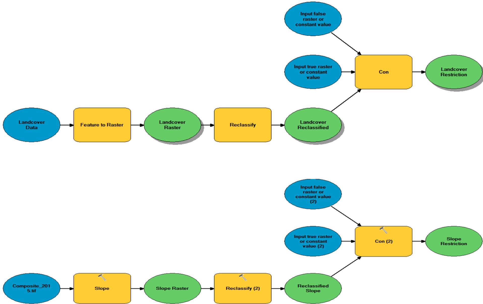
**Fig 5a Site Screening Models for Land Cover/Use, Slope and Similar Area-based Criteria**
