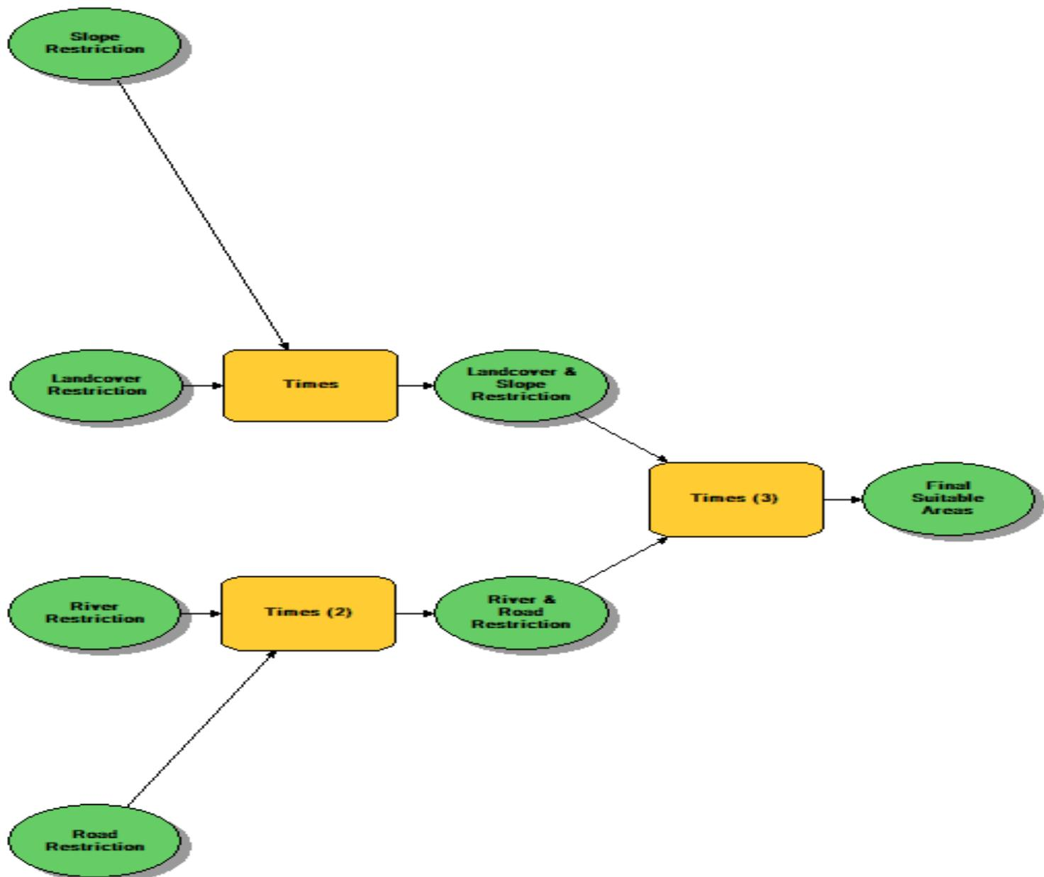
**Fig 5c Integrated Site Screening Model for Mixed Classes of Feature-based Criteria**
