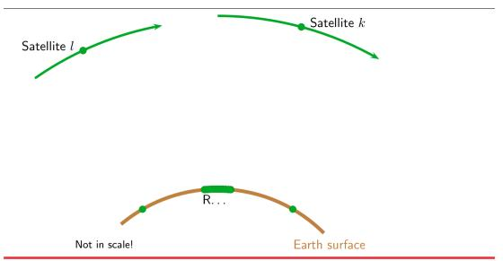
$$L_1^k = \left| \vec{x^k} - \vec{x_1} \right| + T_1^k + c\delta_1 - c\delta^k + \lambda N_1^k \qquad L_1^l = \left| \vec{x^l} - \vec{x_1} \right| + T_1^l + c\delta_1 - c\delta^l + \lambda N_1^l \qquad .$$
