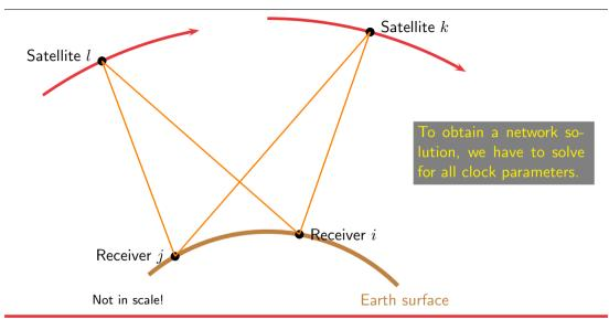
$$L_i^k = \left| \vec{x^k} - \vec{x_i} \right| + T_i^k + c\delta_i - c\delta^k + \lambda N_i^k \qquad L_i^l = \left| \vec{x^l} - \vec{x_i} \right| + T_i^l + c\delta_i - c\delta^l + \lambda N_i^l \qquad .$$
