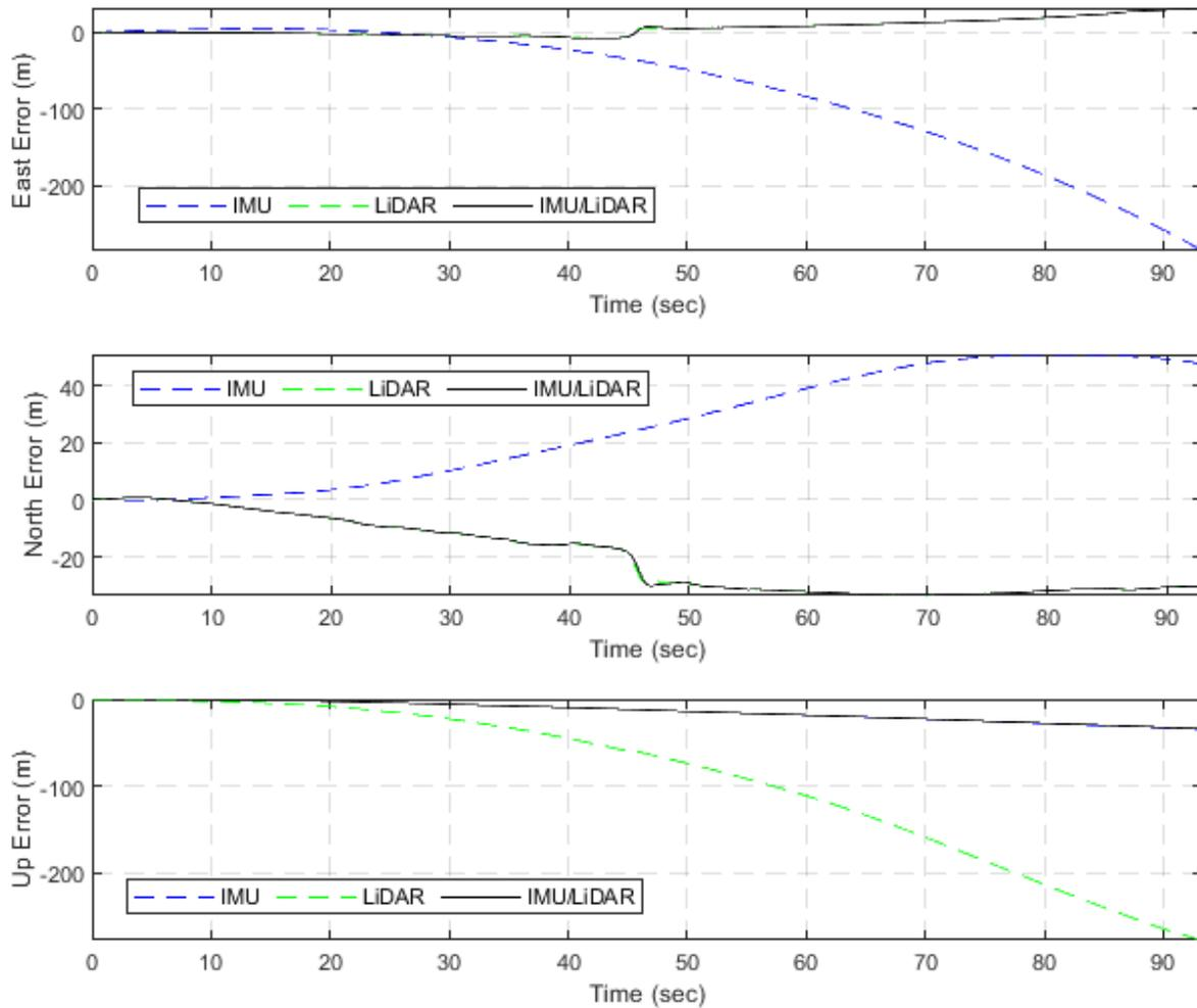
Figure (4): Highway dataset - complete GNSS signal outage: position errors (ENU)
