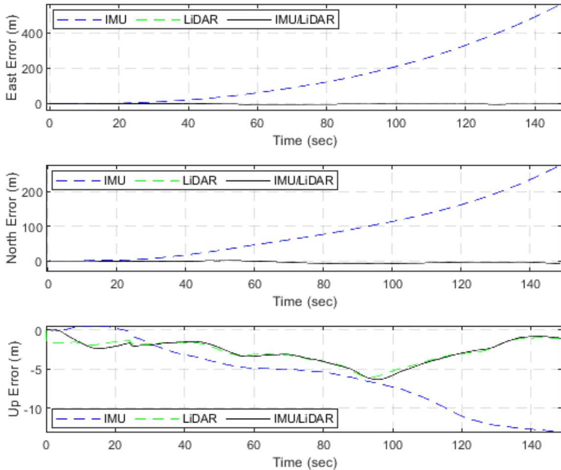
Figure (2): Residential dataset - complete GNSS signal outage: position errors (ENU)
