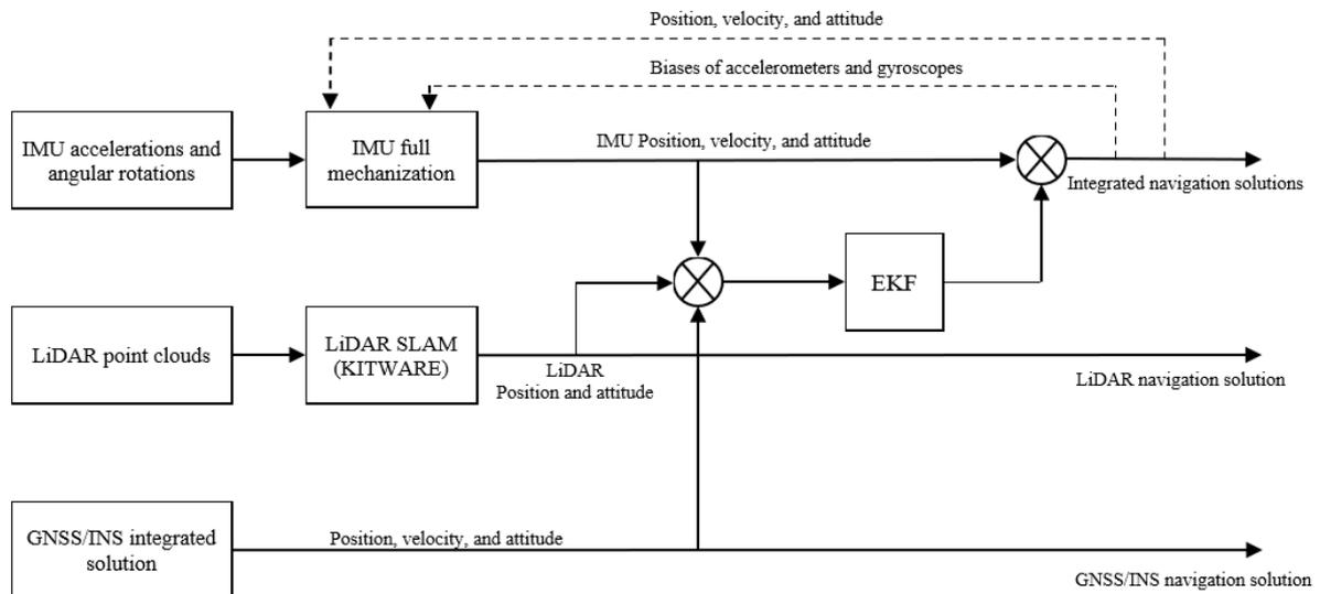
Figure (1): A block diagram for the GNSS/LiDAR/IMU LC integration
