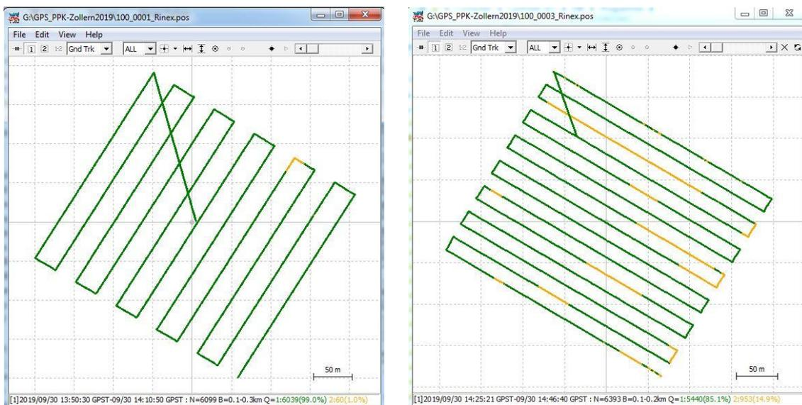
Fig 10: Share of FIX (green) and FLOAT solutions (yellow) from post-processing with RTKLIB for flights with system D (flight altitude above ground, left 50 m, right 60 m)
