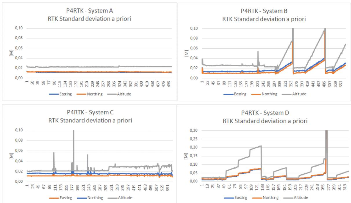
Fig. 4: Standard deviations (à priori) of the image positions determined by RTK (measured EO) of the Phantom 4 RTK systems A - D.
