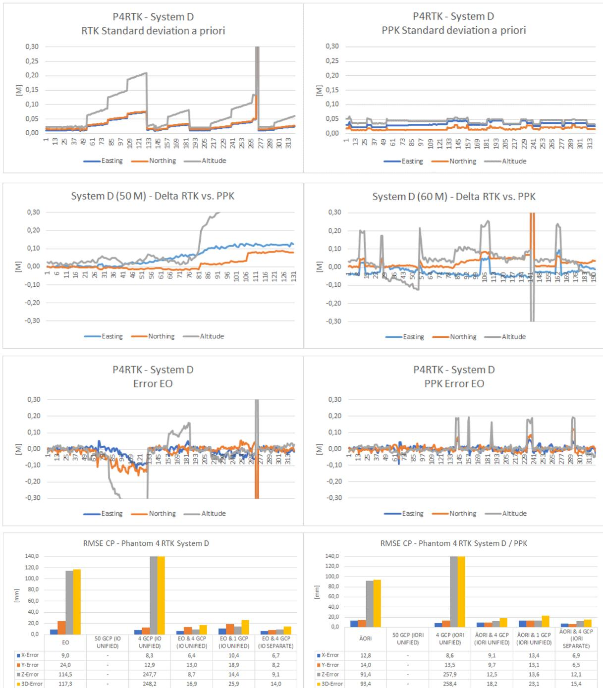
Fig. 9: Comparison of evaluations based on RTK (left) and PPK (right) for system D:
