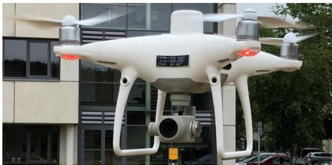
Fig. 1: DJI Phantom 4 RTK
