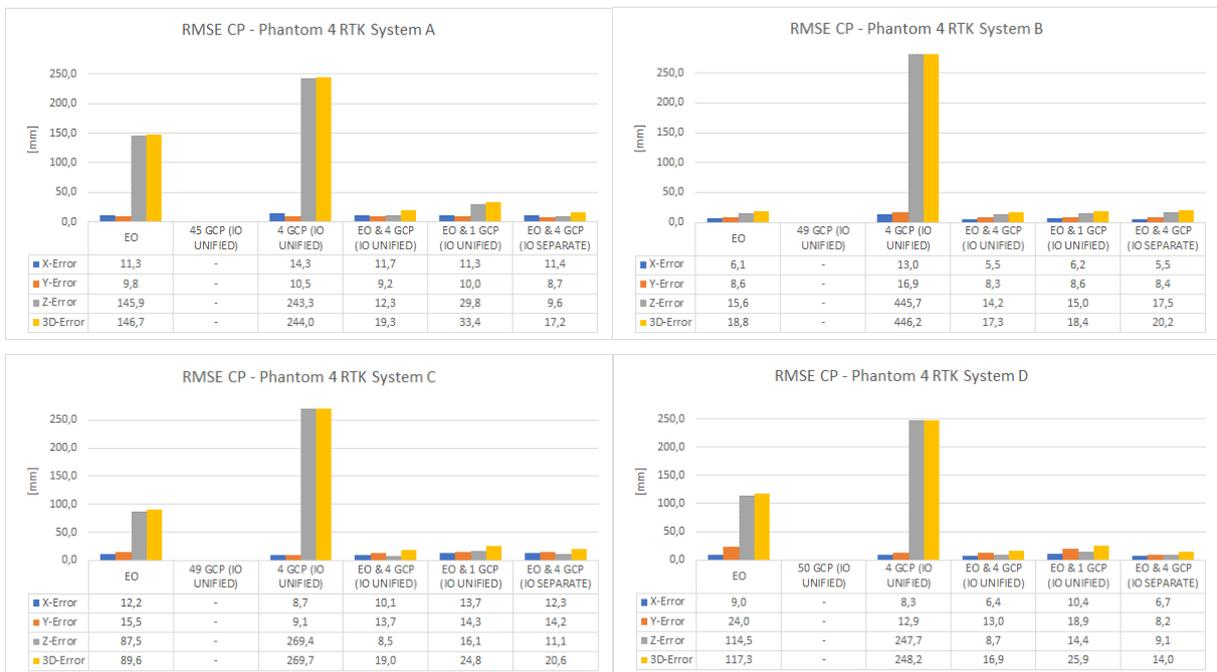
Fig. 7: RMSE values at the control points (CP) as a function of the orientation type (direct: EO – indirect: GCP – integrated: EO+GCP) (systems A - D). Note: the vertical scaling differs from that of GCP (Fig. 6) by a factor of 10.
