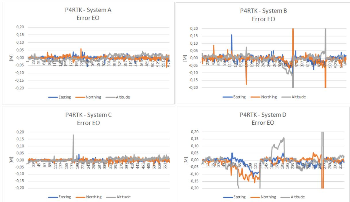
Fig. 5: Residuals (Error) at the image positions determined by RTK (EO) after the BBA for the systems A - D
