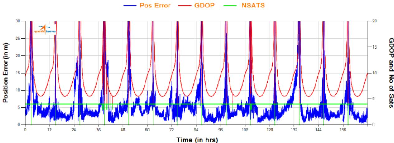
Position Error with Single Frequency Receiver (S-band with Grid Model for Ionospheric Correction)
