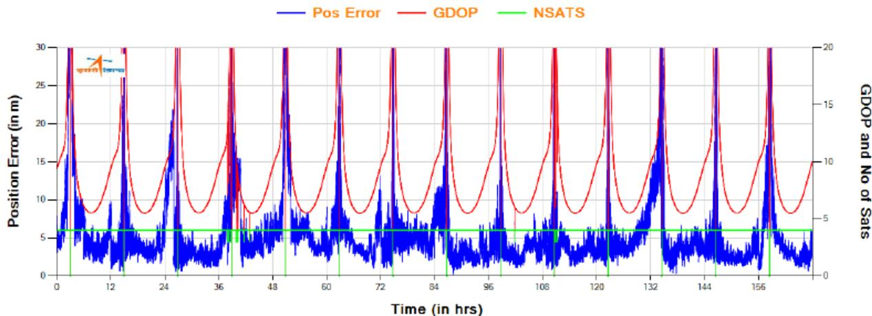
Position Error with Dual Frequency Receiver (L5 and S band)
