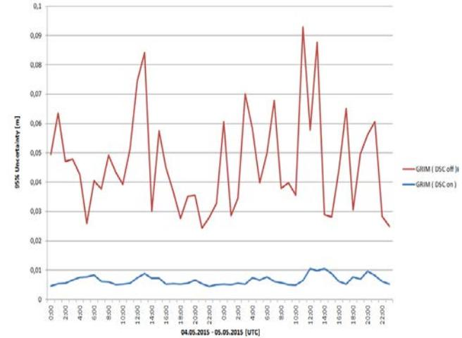
**Figure 8: Predicted geometric error for RTX Net Processor, with DSC disabled and enabled**
