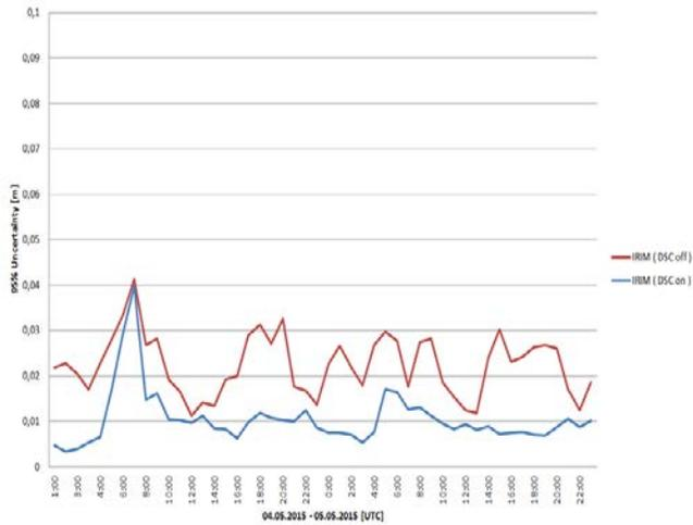
**Figure 5: Predicted ionospheric error for Network Processor, with DSC disabled and enabled**
