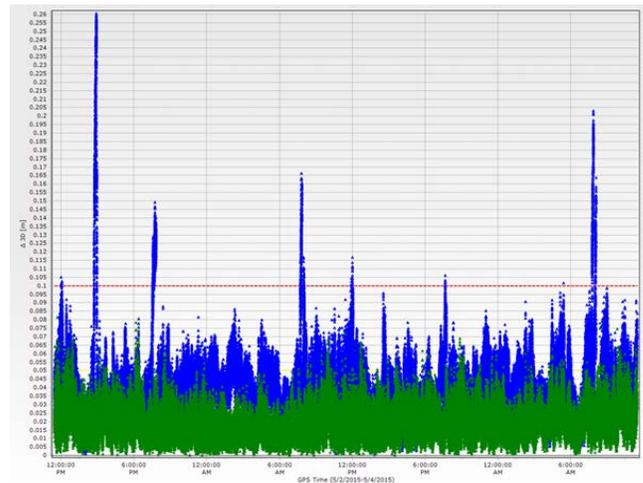
**Figure 9: Rover position scatter plot when using corrections from a network of reference stations using network processors with DSC disabled (blue) and DSC enabled (green)**
