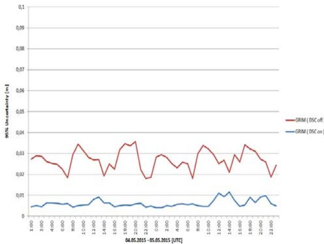
**Figure 6: Predicted geometric error for Network Processor, with DSC disabled and enabled**
