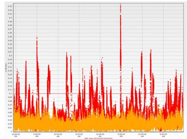
**Figure 10: Rover position scatter plot when using corrections from a network of reference stations using RTXNet processors with DSC disabled (red) and enabled (orange)**
