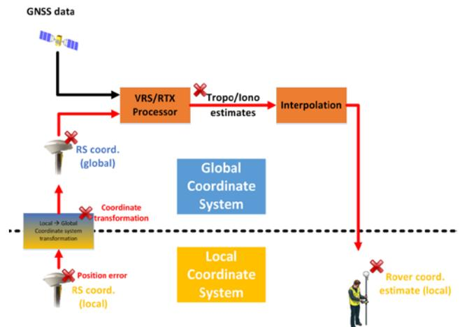
**Figure 2: Rover coordinate estimation using Reference Stations with the traditional approach**
