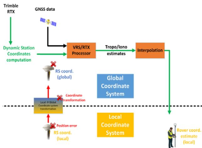
**Figure 3: Rover coordinate estimation using Reference Stations with the DSC approach**
