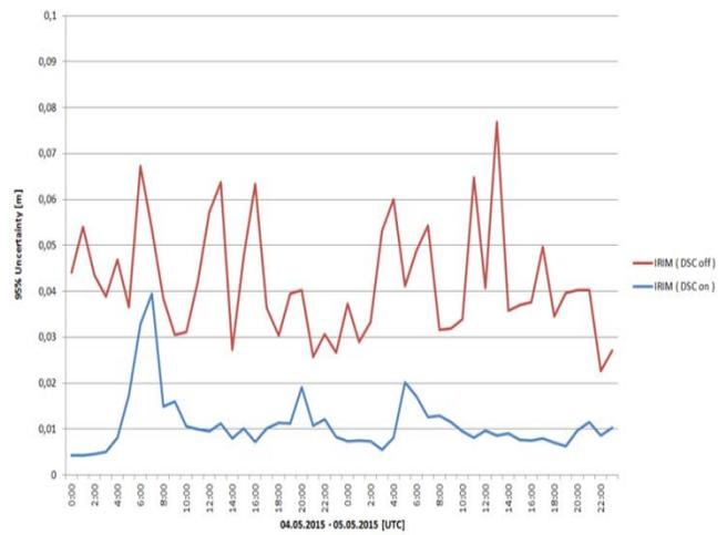
**Figure 7: Predicted ionospheric error for RTX Net Processor, with DSC disabled and enabled**
