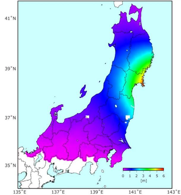
Correction parameters were calculated mainly from GEONET and applied for about 44,000 triangulation control points
