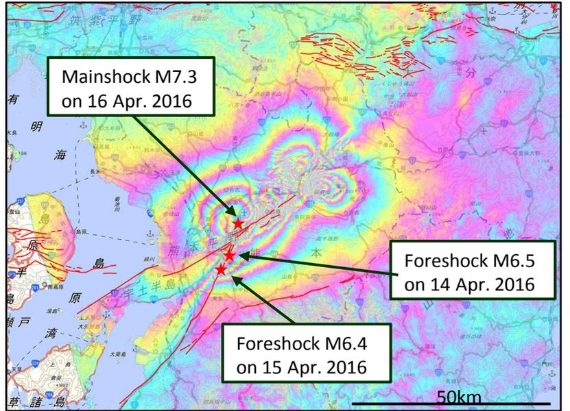
Displacement detected by ALOS-2 InSAR
