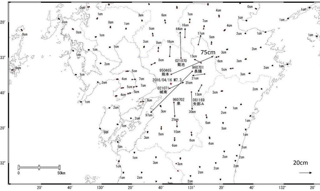
Horizontal displacement detected by GEONET
