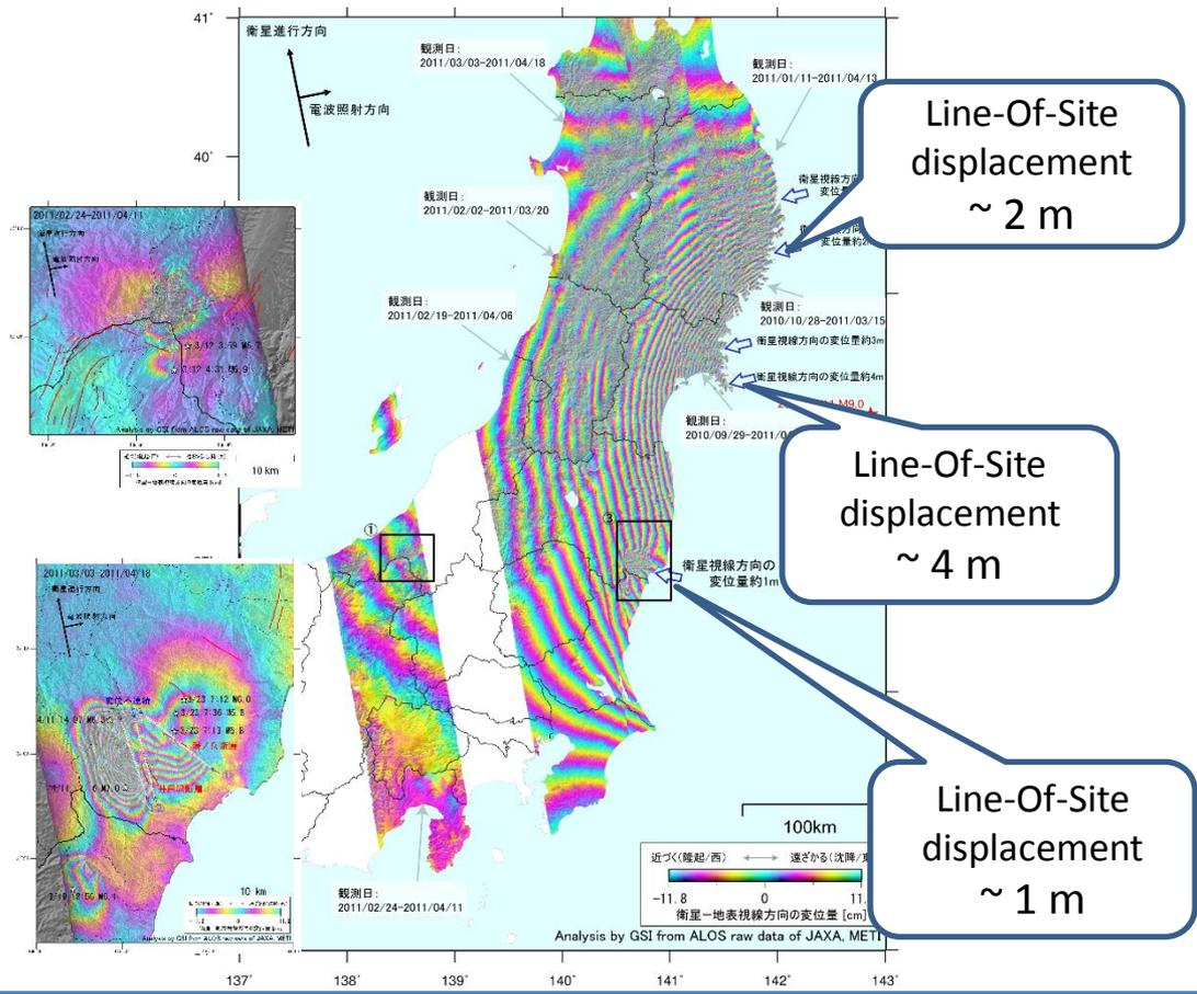
InSAR detected the deformation of magma chambers beneath volcanoes (Takada & Fukushima, 2013)
