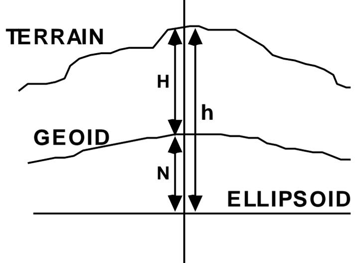
The geoid is modelled by the ellipsoid, with  $a, f$  - (geometry) and  $GM, \omega$  - (physical properties)
