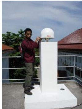
Figure 6. The antenna of Leica AT 504 Choke Ring belongs to Geodetic Dept., UGM CORS which has been installed at the top of Geodetic Department, UGM, Yogyakarta.
