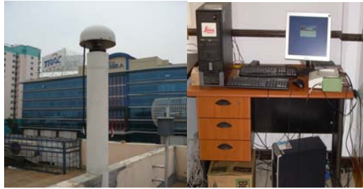
Figure 4. Antena GPS type AT 504 Dorne Margolin (left) and Receiver GPS Leica GRX1200 dan PC Serve (right), Koesoema (2008)
