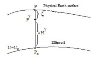
Fig.1. The Satellite system of normal heights
