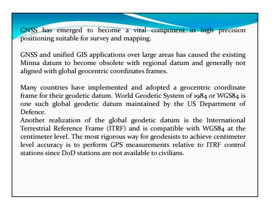
All modern GNSS use geodetic reference systems closely aligned with ITRF (e.g. the US GPS system's WGS84), with few millimeters and forms a robust basis for any regional or national geodetic datum.
