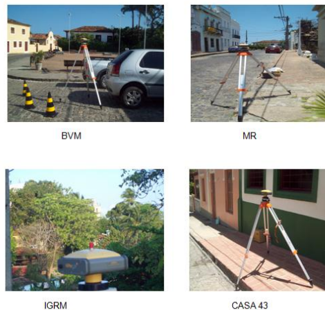
Figure 7 - GNSS occupation of the reference points: BVM, MR, IGRM and HOUSE 43. Photos: November 2010. Source: SOUZA (2012).
