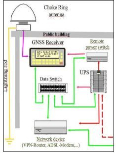
Fig. 4 Scheme of GNSS permanent station
