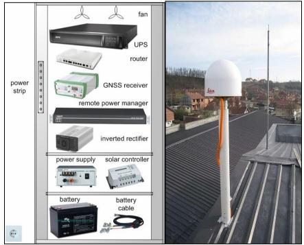
Fig. 5 Equipments pleased in the cabinet and the GNSS antenna in one of the stations
