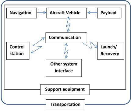
Figure 1 UAV system component
