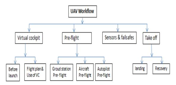
Figure 2 Unmanned Aerial Vehicle workflow.
