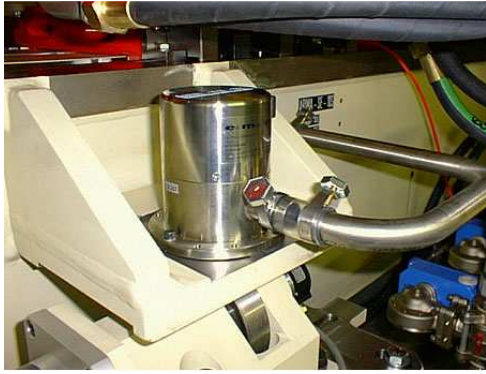
Fig. 7a): Level sensor mounted on the girder, and connected to the stainless steel piping system.
