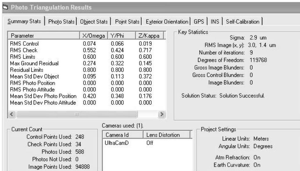
Figure 4 - Aerotriangulation results.
