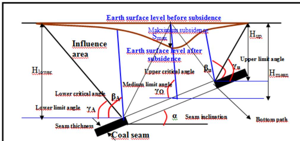
Figure 1. Subsidence tub forming after production in inclined coal seams and the other related definitions (Kratzsch, 1983).
