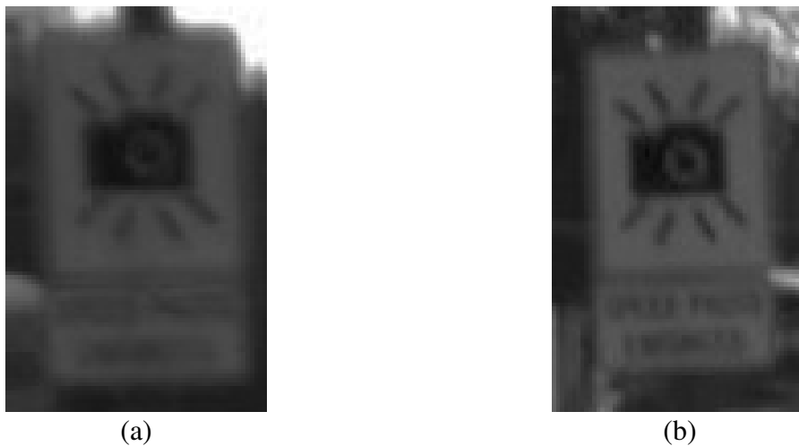
Figure 8: Difference of sharpness of the two cameras: (a) camera 1 – left; (b) camera 5 – right.
