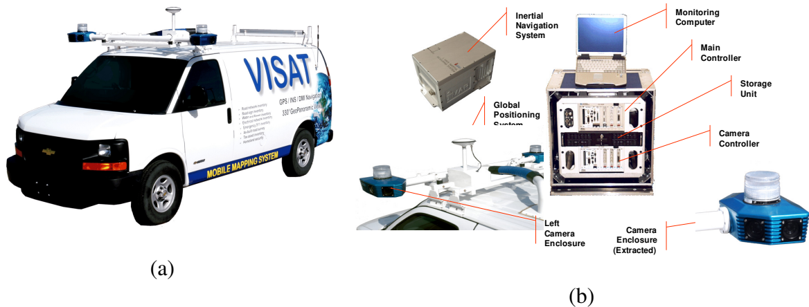
Figure 1: (a) VISAT™ Van (Absolute Mapping Solutions), (b) system components.
