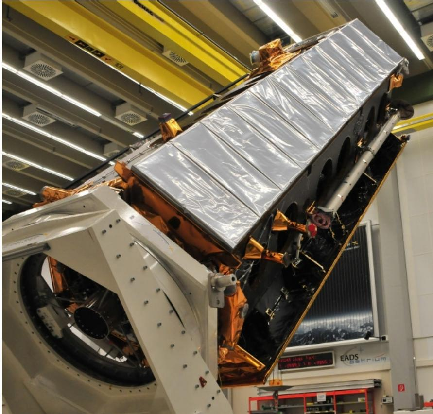
*Fig. 2: SAR panel of TanDEM-X satellite*
